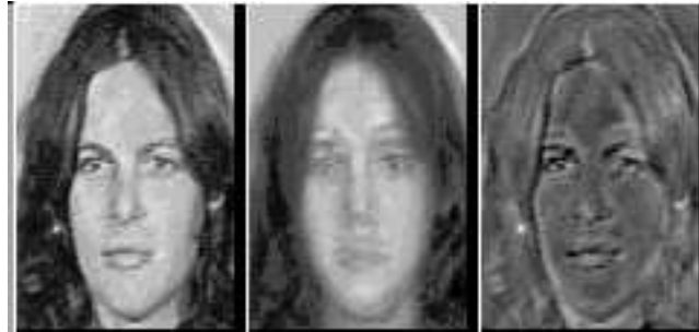
Fig. 1. An illustration of the identity-specific information in faces, using principal component analysis [1]. The original face appears on the left. The middle image is a reconstruction of the face using the first 40 eigenvectors. The rightmost image is reconstruction of the face with all but the first 40 eigenvectors. As can be seen, it is much easier to identify the face when it is reconstructed with eigenvectors with relatively smaller eigenvalues.
